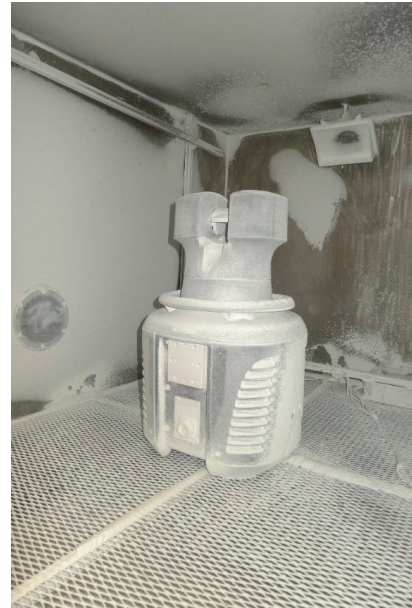
Fig. 11 APDIS after IP5X test.
