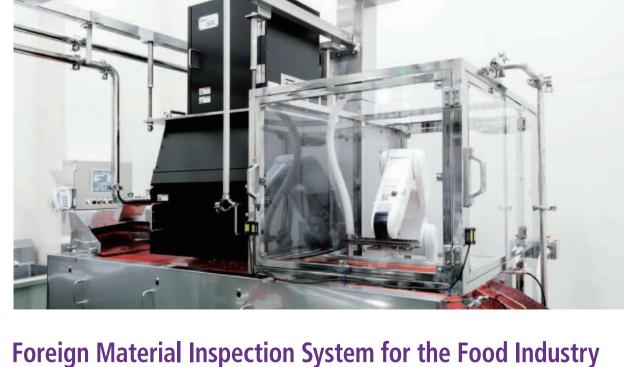
Uses spectroscopic technology and AI to detect organic substances. (Foreign material inspection system for jam and fruit spreads developed jointly with AOHATA Corporation to enable automatic inspection of foreign material and impurities in the jam and fruit spread manufacturing process)
