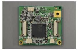
Printed circuit board for land surveying equipment
