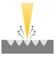
Capable of forming micron-sized riblets
