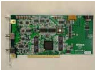
Image processing board for a confocal microscope
