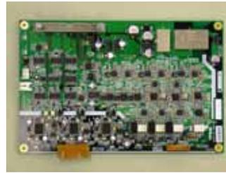
Motor control board for an immersion scanner
