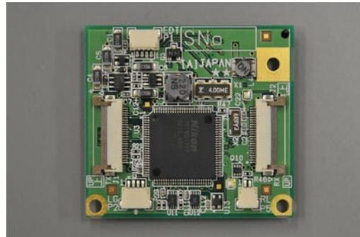
Printed circuit board for land surveying equipment
