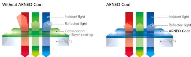
Fig. 3 Difference between conventional coat and ARNEO coat.
