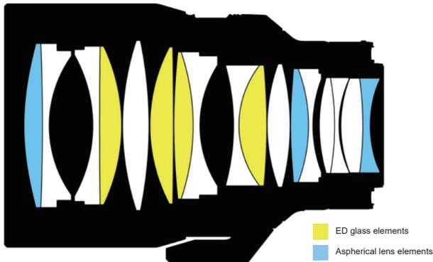
Fig. 2 Lens configuration diagram.
