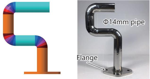
Fig. 13 Sample of pipe modeling with five-axes.
