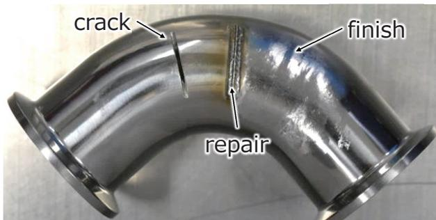
Fig. 12 Repair of damage in a pipe.
