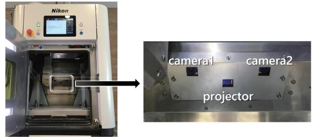
Fig. 4 Built-in stereoscopic phase shift 3D scanner
