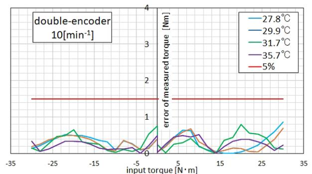
Fig. 13 Temperature-torque error characteristics (double encoder)
