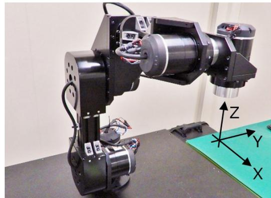
Fig. 9 Articulated robot (payload: 5 kg) for accuracy evaluation
