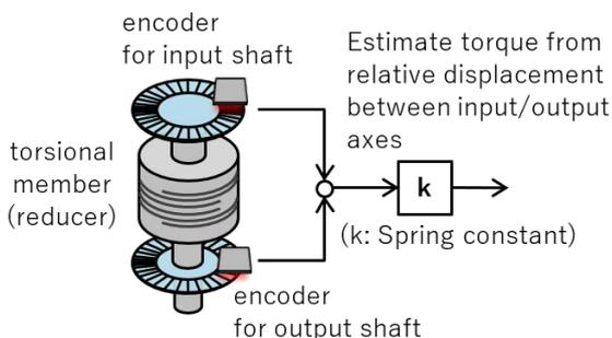
Fig. 5 Double-encoder arrangement
