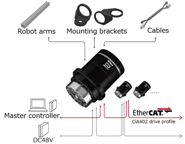
Fig. 3 System configuration
