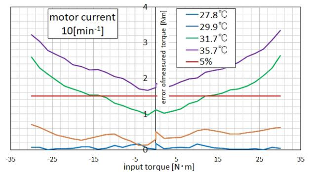
Fig. 12 Temperature-torque error characteristics (motor current detection)
