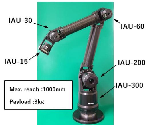
Fig. 4 Example of 5-axis robot using C3 eMotion
