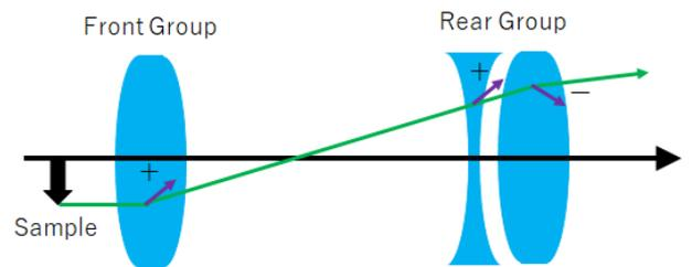
Fig. 3 Power configuration of high-magnification objective lenses
