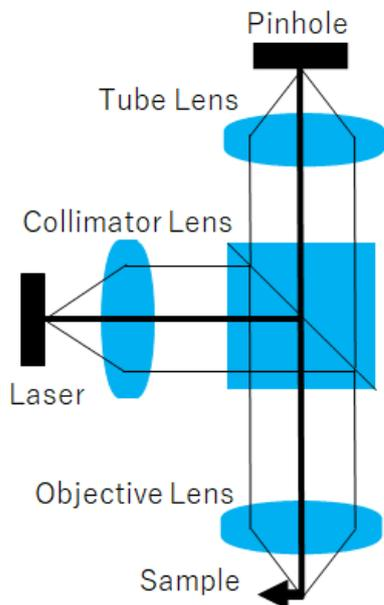
Fig. 4 Schematic of the confocal laser scanning microscope
