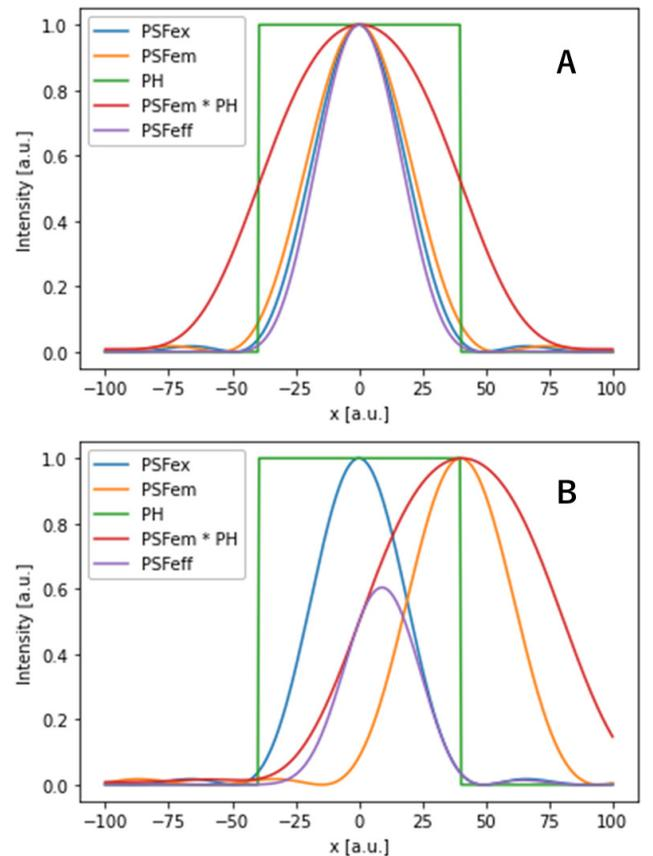
Fig. 5 Effective Point Spread Function of confocal laser scanning microscope  $PSF_{eff}$
