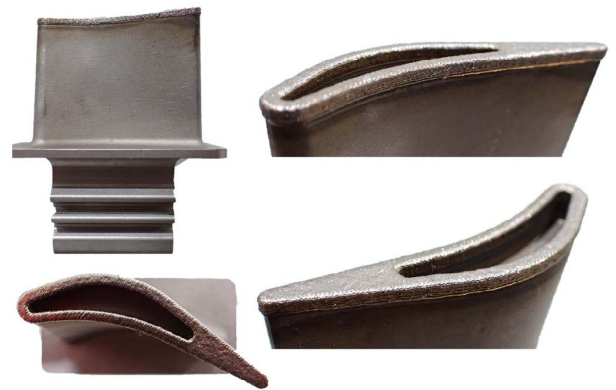
Fig. 10 Turbine blade tip repair
