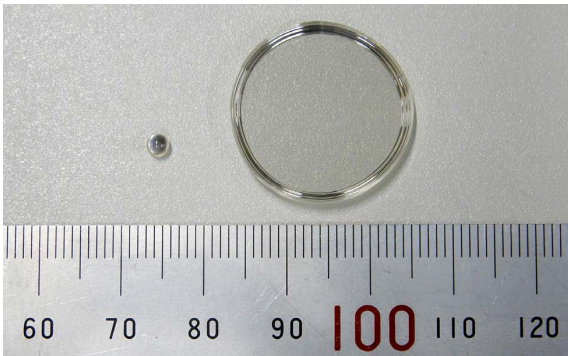
Fig. 1 Photograph of LT (left, 2.8 mm in diameter) and LTZS (right, 23 mm in diameter): LTZS is polished into disk (3 mm thickness) for the optical property measurement.
