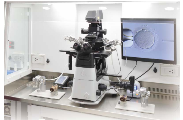
Fig. 9 Example setup of an inverted microscope
