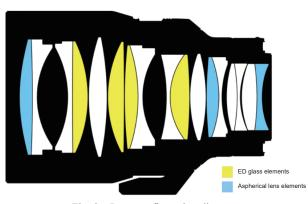
Fig. 2 Lens configuration diagram.
