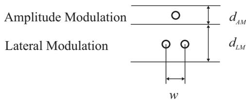
Fig. 3 Schematic diagram of the dual-layer haptic button. The depth  $d$  of each layer indicates the region where the AM or LM stimulus is presented.  $w$  indicates a value twice that of the LM vibration amplitude.
