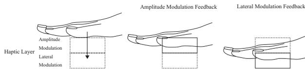
Fig. 1 Midair click using dual-layer haptic feedback. The intensity and quality of haptic feedback are switched according to the hand position.
