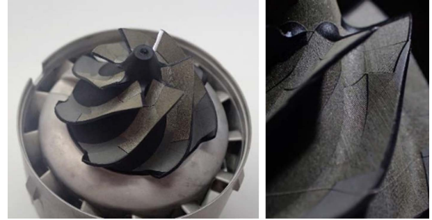
Fig. 5 Riblet processing on a 3D curved surface
