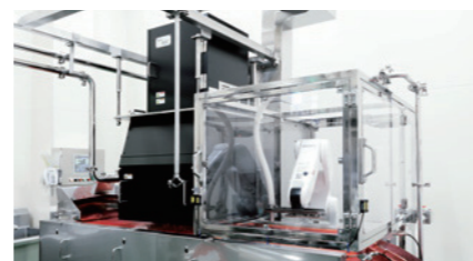
Foreign Material Inspection System for the Food Industry Uses spectroscopic technology and AI to detect organic substances. (Foreign material inspection system for jam and fruit spreads developed jointly with AOHATA Corporation to enable automatic inspection of foreign material and impurities in the jam and fruit spread manufacturing process)
