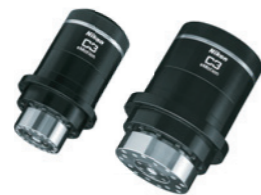
Intelligent Actuator Unit "C3 eMotion" A joint unit for a collaborative robot that integrates a motor, speed reducer, driver, brake and encoders.
