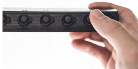
Mockup to test the angles of backside buttons
