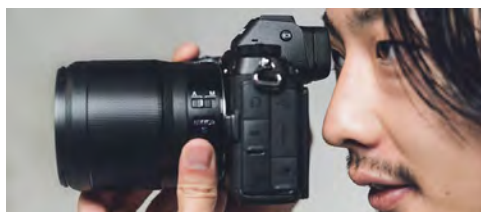
EVF that prevents the nose from contacting with the LCD screen using a protrusion at the back
