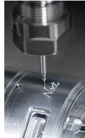
Fig. 5 “Noct” character engraving process.
